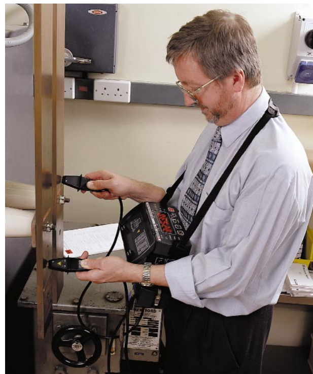
The DLROs are light enough to be worn around the neck. They are also small enough to be taken into areas which were previously too cramped for easy testing.
