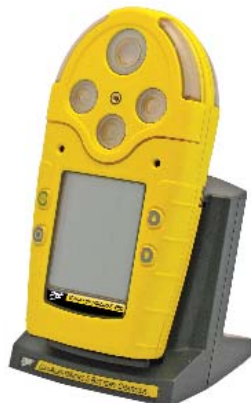
Optional rechargeable battery and slip-in cradle charger
