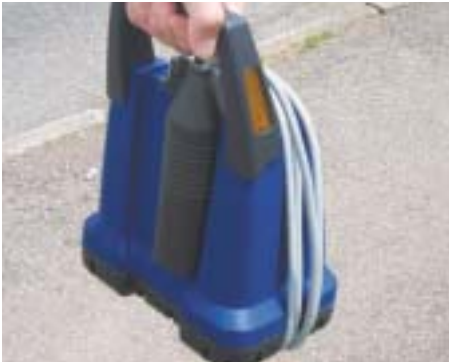
Outstation design incorporates sensor storage and cable wrap
