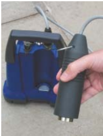
New digital sensor with enhanced low frequency sensitivity
