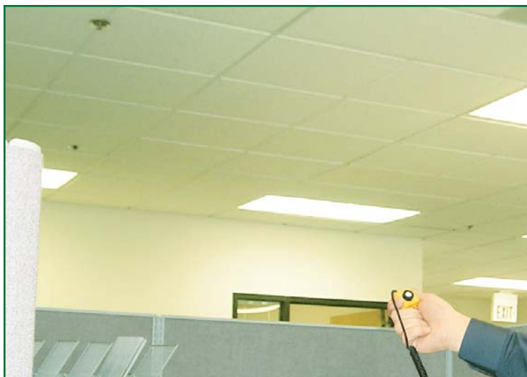
Removable light sensor makes it easy to accurately measure lighting in office environments. The probe may be extended to avoid shadowing and may be oriented towards a specific light source.
