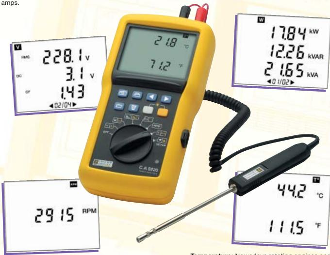
Rotation speed: For predictive maintenance, it is necessary to regularly test rotation speed on rotating machines. The C.A 8220, an all-inone instrument, meets this requirement simply and effectively. ■ Temperature: Nowadays rotating engines and machines are equipped with temperature probes that are easily accessible on a terminal board. By simply connecting the C.A 8220 to this terminal board, it is possible to directly measure the engine's internal temperature.
