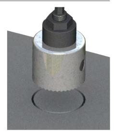
To score coatings thinner than 0.5 mm (20 mils), a sharp knife may be sufficient to carefully score around the dolly once it has been secured in place by adhesive.
