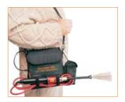
Available in 2 versions, 15kV and 30kV, each Elcometer 236 unit provides the user with complete control of voltage and sensitivity settings.
