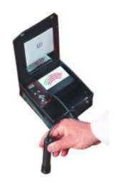
The ETI 7000 general purpose moisture meter combines the scales of both timber and building moisture meters. The instrument is housed in an ABS case within a custom-made carrying case. The ETI 7000 incorporates a clear analogue meter which has five colour-coded scales:- wood 1, wood 2, plaster, concrete and a reference scale. The reference scale is calibrated 1 to 10 and is used to take comparison readings without reference to moisture % content.
