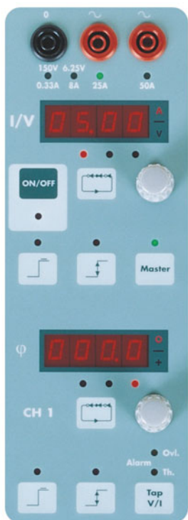
Current / voltage channel
