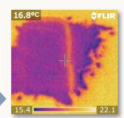
The thermal image clearly shows moisture in a floor. Something which can not be detected by the naked eye.
