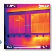
The occupant complained about a cold spot in his living room. The thermogram on the right clearly identifies the source of the cold as an uninsulated part in the wall. By insulating this spot, the occupant improved comfort, saved energy and money.
