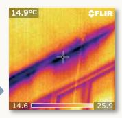
The thermal image shows a badly sealed ceiling causing cold air to leak into the building.
