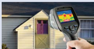
Infrared cameras quickly locate moisture related problems
