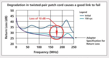
As you can see in this graph, a commercial Cat 7 SSTP cord has a 10 dB loss after 150 cycles of coiling and uncoiling. This 10 dB degradation causes a good link to fail – and you end up with a false fail. This 10 dB of loss won't occur when you use Fluke Networks' Permanent Link adapter technology – with DTX you get repeatable accuracy you can count on.
