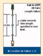
whether the problem has been resolved – the technician knows exactly where to look and what to do to fix the failing link. Even if only two percent of the cables certified in one shift fail Autotest, you'll save as much as two hours of labor time per day of certifying.
