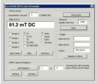
A full driver suite is available as an optional extra. This includes sample programmes with full source code (Microsoft Visual C++.NET) for the 2000 operating system, XP and later. A simple DLL allows third party integration of the GMO8 into embedded systems. A labview VI is included. Linux is also supported.
