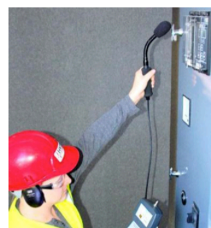
Optional Indoor Acoustic Probe (PDSIAP) in use with Headphones. Outdoor Parabolic Receiver (PDSOPR) also available.
