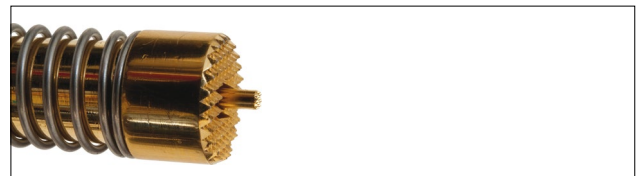
The "double" probe tip showing the springy center tip
