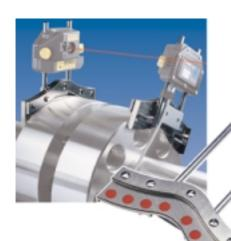
Shafts can't be rotated? No problem with ROTALIGN® PRO! Simply place the ALI 2.230 magnetic sliding bracket onto the coupling flange or shaft end and slide it around the circumference to take measurements in seconds. Suitable for shaft/coupling diameters from approx. 80 mm (3 1/8") on up.
