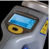
In the R mode the C.A.T<sup>3</sup> detects VLF radio signals re-radiated by buried metallic pipes and cables.
