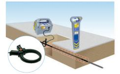
SIGNAL CLAMPING (Optional) Applies a Genny<sup>3</sup> signal safely to a pipe or live cable up to 76mm diameter without interrupting the supply.
