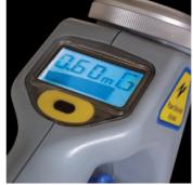
In the G mode the C.A.T<sup>3</sup> detects a tone radiated by the Genny+ to a buried conductor.
