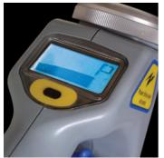
In the P mode the C.A.T<sup>3</sup> detects 'power' signals that are being radiated by loaded cables.
