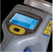
In the R mode the C.A.T<sup>3</sup> detects VLF radio signals re-radiated by buried metallic pipes and cables.
