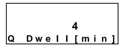
Use the UP or DOWN arrow to set the dwell time. In the above example, the HygroPalm AW1 will wait 4 minutes before processing the humidity data with the AwQuick algorithm.
