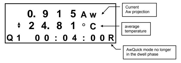
When the projected value of Aw is stable, the HygroPalm AW1 freezes the display. Black rectangles to the left of the display indicate that the measurement is ended.
