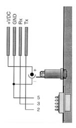
Power supply, 3.5mm Jack female AC adapter 12 to 15 VDC, 100 mA
