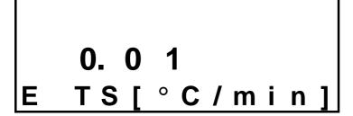
Use the UP or DOWN arrow to set the definition of stable temperature. In the above example, the HygroLab will consider temperature to be at equilibrium when the rate of change of the temperature signal is less than  $0.01~^{\circ}$ C per minute. Default value:  $0.01~^{\circ}$ C / min
