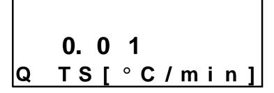
Use the UP or DOWN arrow to set the definition of stable temperature. In the above example, the HygroPalm AW1 will consider temperature to be stable when the rate of change of the temperature signal is less than 0.01 °C per minute.
