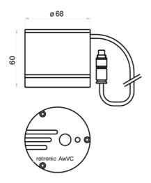
Both probes are physically the same with the difference that the AwVC-DIO incorporates a small fan to ventilate the product sample. This can be beneficial when measuring chunky product samples.
