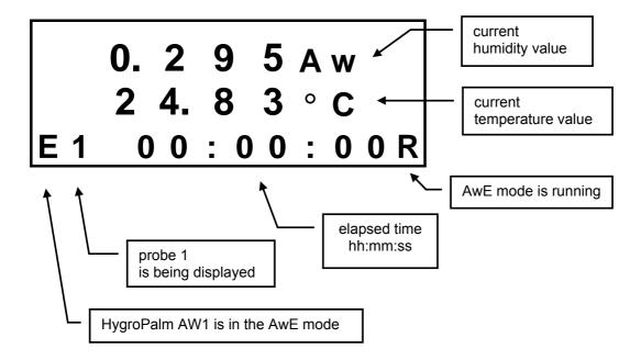
After 60 seconds, the trend indicators appear both for humidity and temperature. Two arrows mean stable signal, as per the settings defined when selecting the AwE mode :
