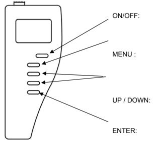
Turns the instrument on or off and also controls the HOLD function. This key has no effect when either the AwQuick or the AwE operating mode is running.
