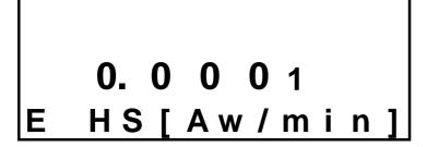
Use the UP or DOWN arrow to set the definition of stable humidity. In the above example, the HygroPalm AW1 will consider humidity to be at equilibrium when the rate of change of the humidity signal is less than 0.0001 Aw per minute. Default value: 0.0001 Aw / min
