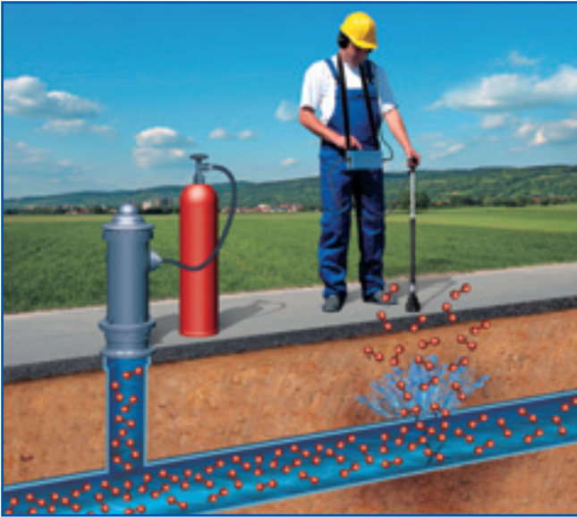
Tracer gas measurement
