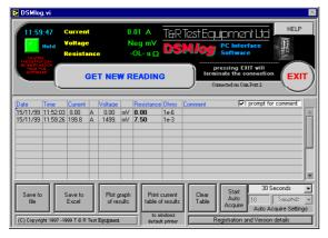
Connecting the DSM200 to a PC running the optional DSM*log* software adds data capture and reporting functions to the unit, allowing test results to be exported directly to Excel or saved to a file. All results are time stamped, and a comment may be added to each test. Data capture can be controlled from the PC, and the resistance of a test object can be monitored over a period of time.
