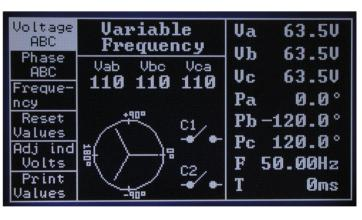
In conjuction with a current source (such as the 200ADM), the DVS3 mk2 can be used to test protection requiring current injection with a phase-shiftable voltage including:
