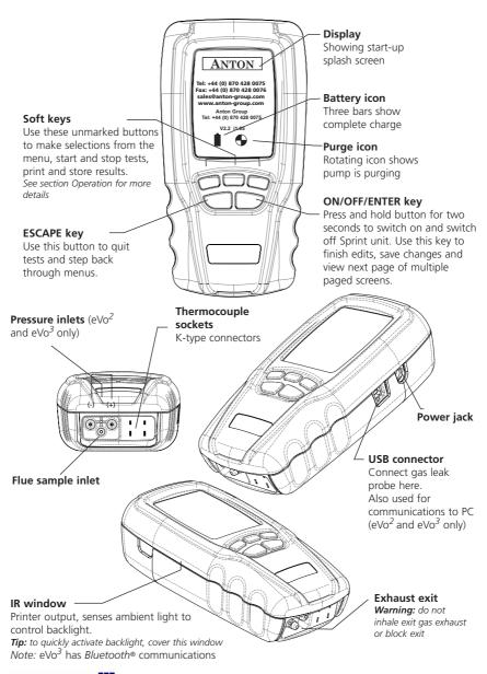
**Tip:** see label underneath unit for details of probe connections. Sprint eVo<sup>1</sup> does not have prssure inlets
