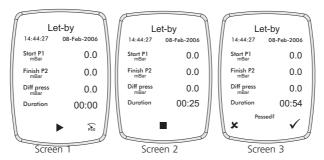
You may fail the test by pressing the key x to indicate test has failed (you can print the results).
