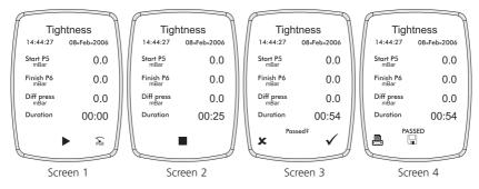
Press the soft key ✓ to pass test.
