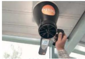
testo 417, e.g. for monitoring the air input at a plate ventilation outlet
