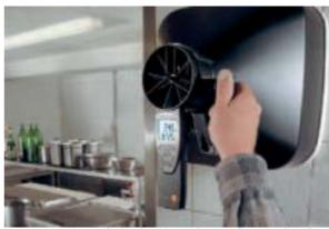
testo 417, e.g. for monitoring the exhaust air at a wall-mounted ventilator
