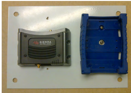
Modem and Protective Boot Secured
