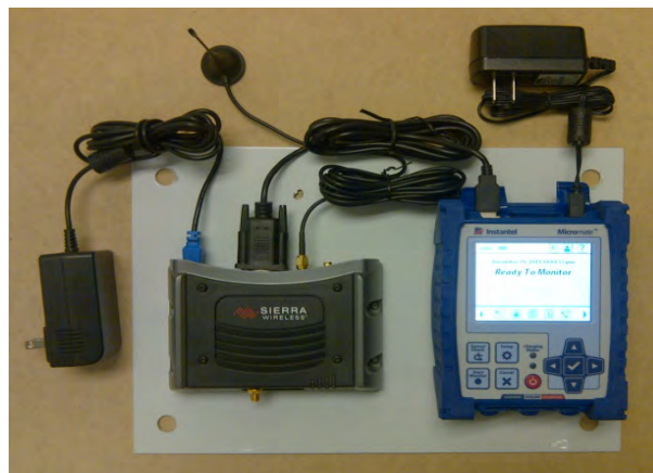
Placement of Modem, Micromate and Cables
