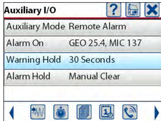
Sample Remote Alarm Setup
