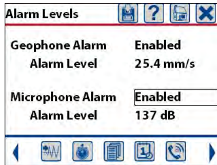
Sample Alarm Source and Alarm Level
