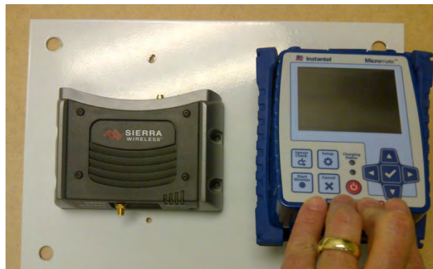
Install the Micromate in the Protective Boot
