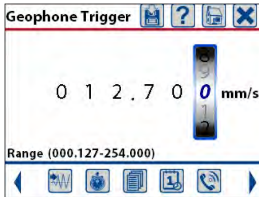
Geophone Trigger Level Set to 12.7 mm/s
