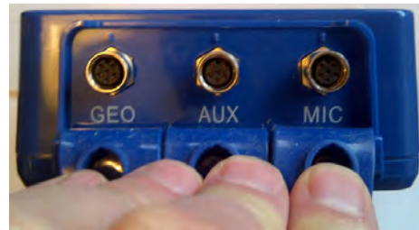
Dust Caps Pulled Back to Access Connectors
