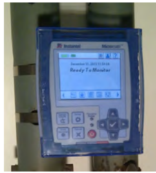
Micromate Attached with Metal Straps
