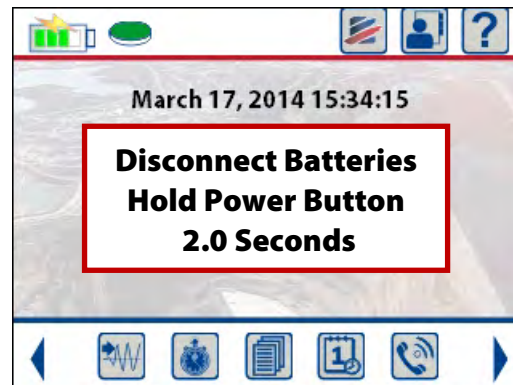
Disconnect Battery Confirmation Message
