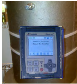
Micromate Attached with Plastic Tie-wraps
