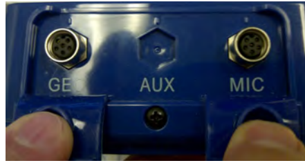
Dust Caps Pulled Back to Access Connectors
