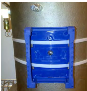
Micromate Attached with Plastic Tie-wraps
