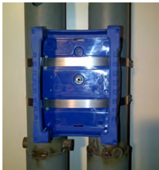
Micromate Attached with Metal Straps
