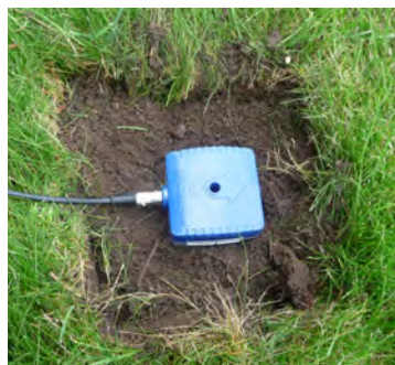
Geophone - Spikes Installed Geophone - Spiked in Ground Geophone - Partially Buried
