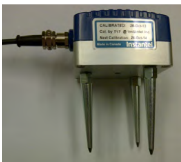
Geophone - Spikes Installed Geophone - Spiked in Ground Geophone - Partially Buried
