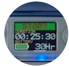
Colour coded display showing remaining battery life
