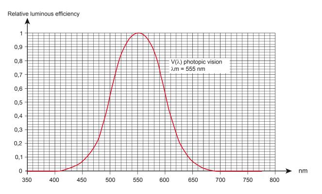
The error on the spectral response of the sensor is equal to the area of the differences between the  $V(\lambda)$  curve and the curve of the sensor.
