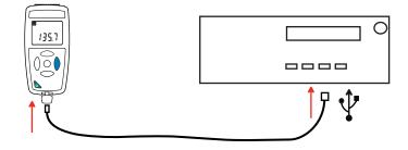
It is treated as a USB key and you can access its content. But to read the records, you must use the Data Logger Transfer software.
