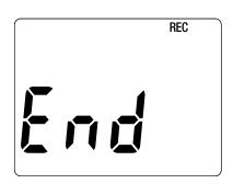
If during start-up the instrument displays the screen shown opposite, it means that a recording session has been brutally interrupted by a power outage.
