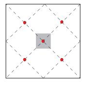
Here's an example of 2 rooms. The represent the luminaires. The • represent the measurement points.
