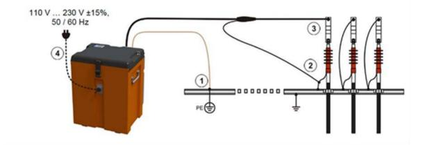
To ensure correct earth connection between return earth (2) and additional safety earth (1), a measurement must be made using an appropriate ohmmeter. The user can then confirm the resistance between earth connections 1 and 2 is no more than 5 ohms. This information is specified in the User Guide.
