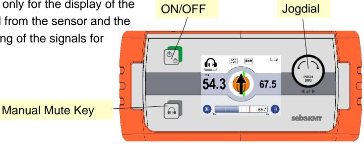
Dimensions (with rubber frame): 65 mm x 225 mm x 100mm (H x W x D)
