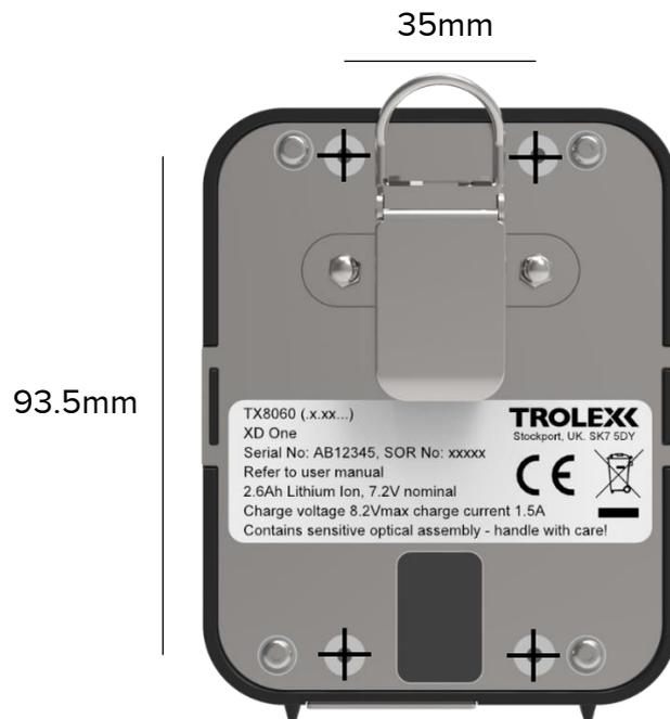
The XD One is supplied with a stability bracket and strap to support the fit of the product when body mounting. Fit the bracket using the bottom two threaded M3 mounting features and the fixing screws provided.
