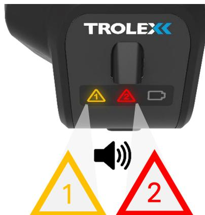
If a threshold is breached during operation, the following alarm sequence is used to alert users to act based on the change in the working environment.
