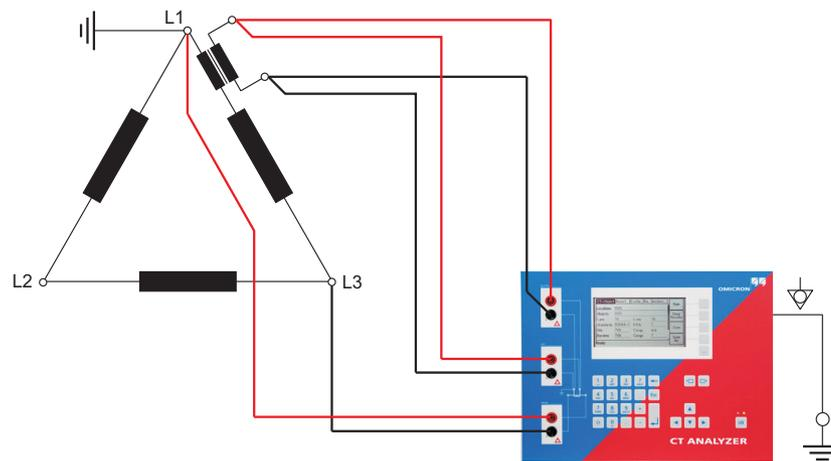
Figure 2-14 Measurement setup for delta compensation "Ratio 2/3"
