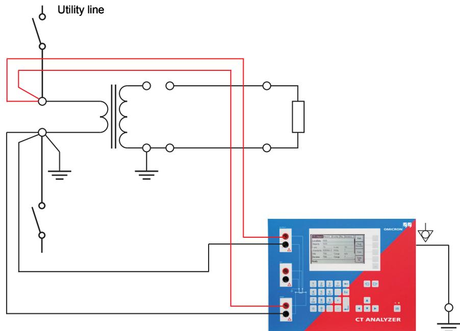
Figure 2-4 Basic wiring for primary winding resistance measurement
