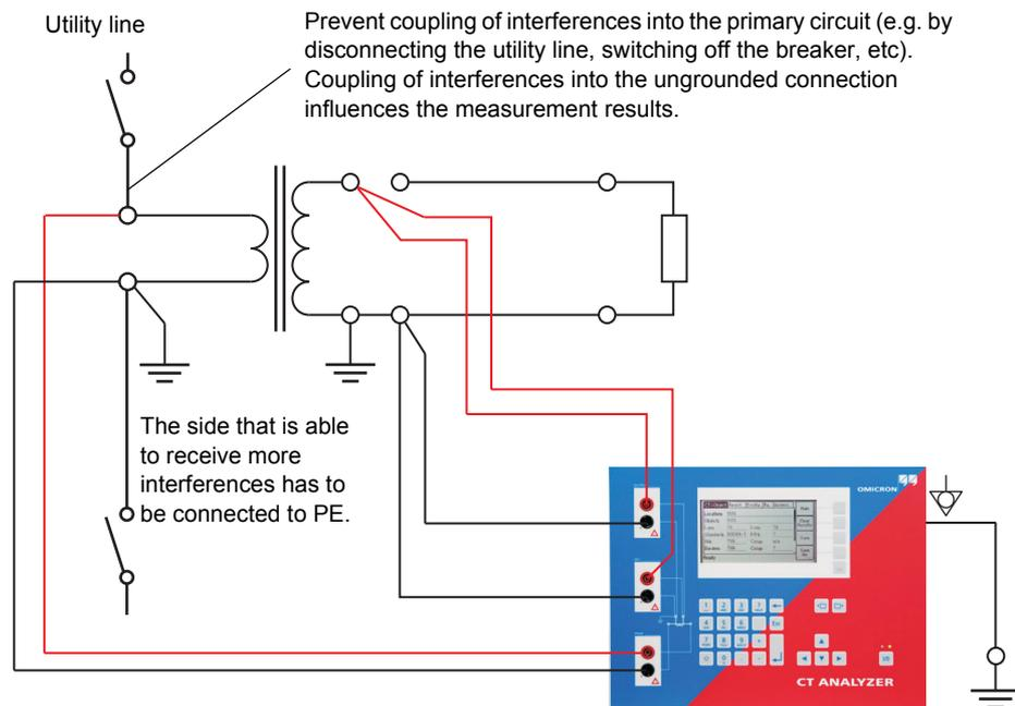
Figure 2-2 Basic wiring for a CT test
