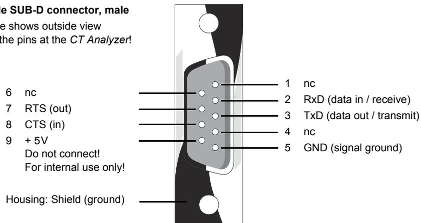
Figure 10-1 Pin assignment for RS232 remote control interface
