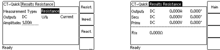
Figure 8-15 **CT-Quick** card and **Results** card for resistance measurement
