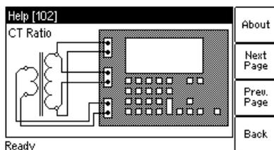
Figure 8-10 Wiring example for CT ratio measurement
