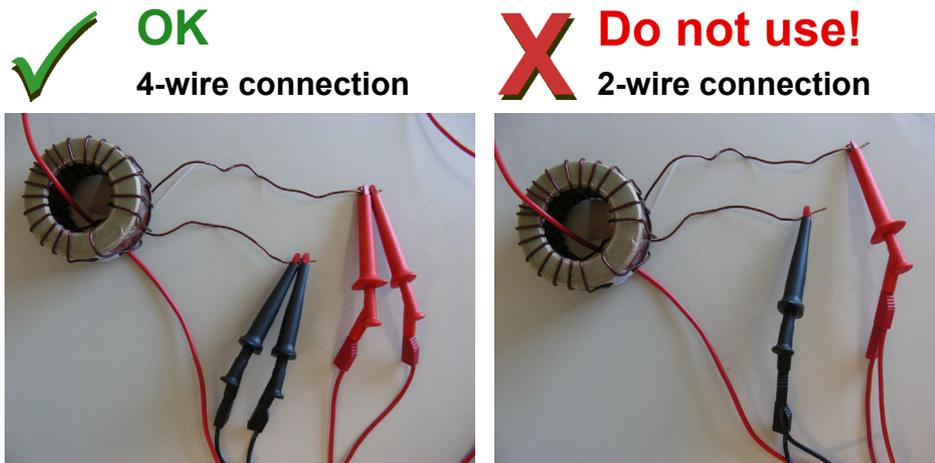
The measurement leads from the "Output" sockets and input "Sec" of the *CT Analyzer* are connected to the test object via separate clamps.
