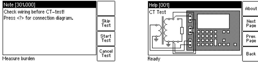
Figure 4-6 CT test: Wiring check message (left) and wiring diagram (right)
