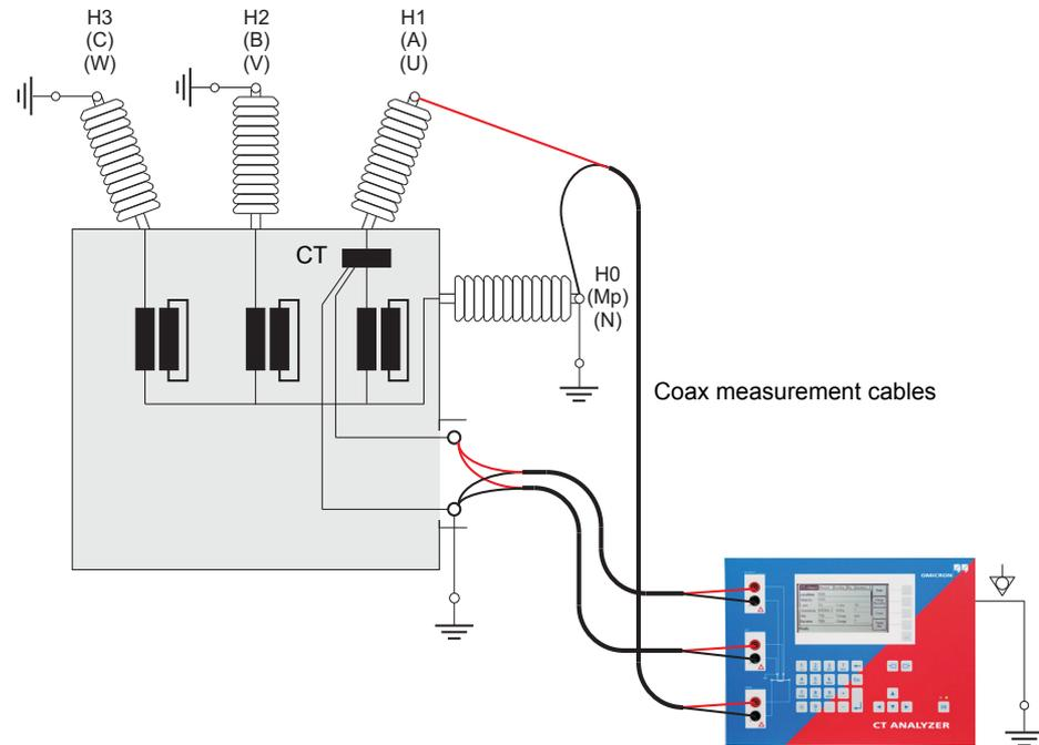
Figure 2-10 Measurement on a bushing-type CT
