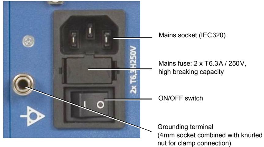
Figure 1-2 Mains connection unit and grounding terminal
