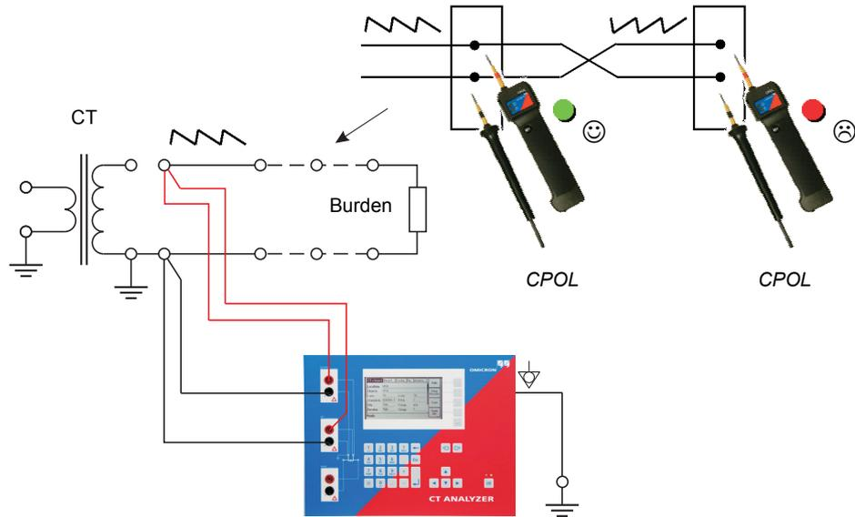
Figure 8-8 Wiring example for polarity check
