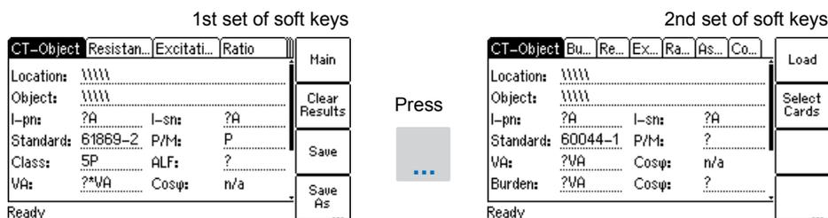
Figure 5-2 Switching the set of soft keys in the CT-Object card
