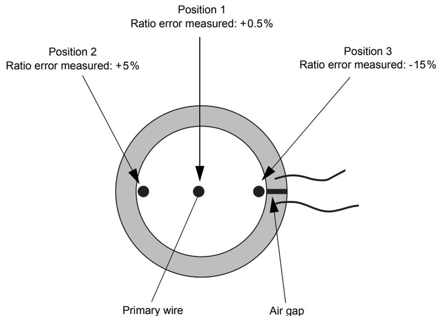
Figure 2-5 Ratio error depending on the position of the primary wire inside the gapped core
