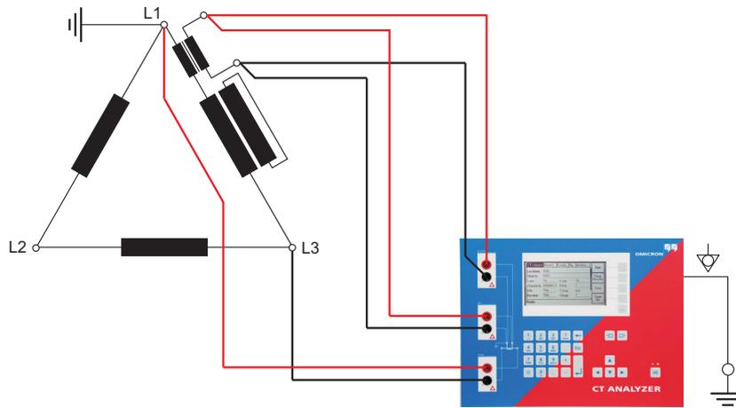
Figure 2-15 Measurement setup for delta compensation "Ratio 1"
