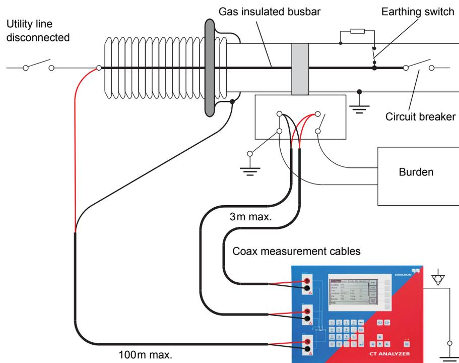
Figure 2-9 Measurement on a GIS (SF6) switch gear
