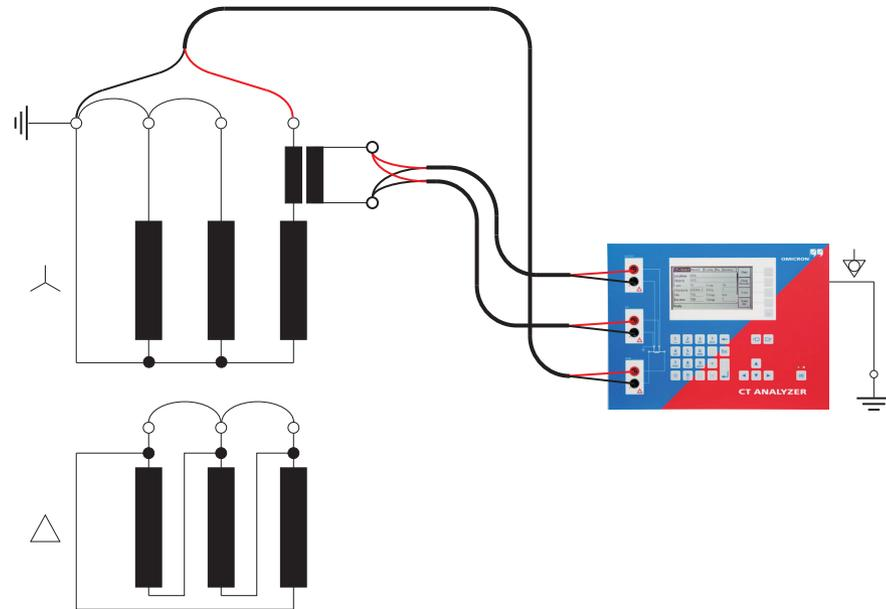
Figure 2-11 Measurement on a Y winding transformer
