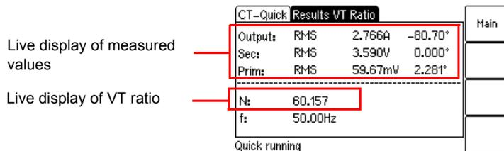
Figure 8-14 **Results** test card for VT ratio measurement
