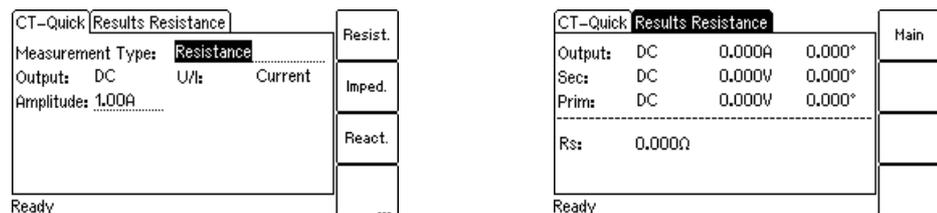
Figure 8-1 **CT-Quick** test card (left) and **Results** test card (right) for resistance measurement
