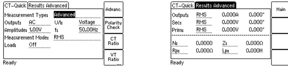
Figure 8-3 CT-Quick card and Results card for Advanced measurement type
