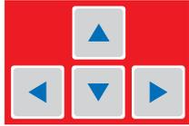
To open the edit mode for a displayed card, press the cursor key. The card's tab is then no longer highlighted (see Figure 5-3). Use the cursor keys to move the cursor and to select the desired edit field. Some edit fields have soft keys assigned. The soft keys available for an edit field are displayed if the field is selected.
