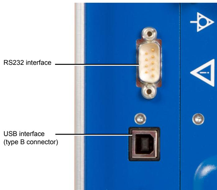
Figure 1-4 Remote control interface (RS232 and USB)
