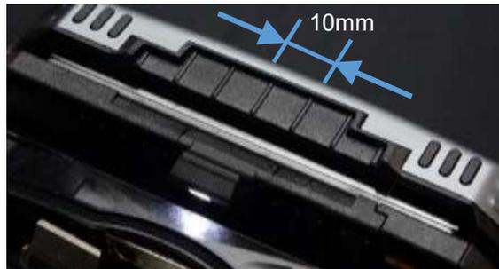
For the 40mm protection sleeve, set the protection sleeve as shown below.
