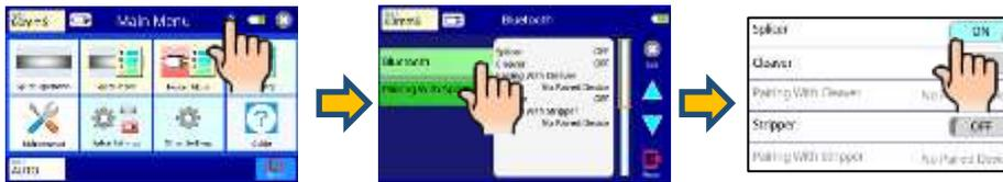
2. Select [Pairing With Splice+] menu and set [Splice+] setting to “ON”.
