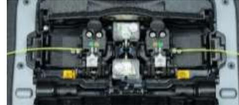
Motion changes by the selected operation mode. When a [Proof test] setup is OFF, sheath clamp will not open after splicing.
