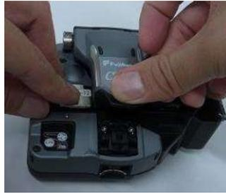
4. Lift the Lever until it stops and remove the fiber from the cleaver. Be careful not to contaminate the end-face of the fiber by touching anything with it.
