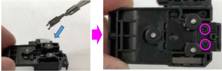
5. Put the big plastic part in the pot of the clamp while keeping pressing down the small plastic part with tweezers.
