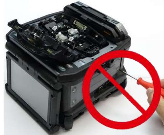
*Do not remove the protector from the fusion splicer, without first consulting a nearest Fujikura authorized distributor for instruction. Tightening the original screw without the protector present may damage mechanism inside.*
