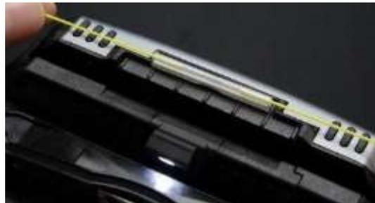
If a protection sleeve is not centered enough, the protection sleeve may not shrink completely as below.
