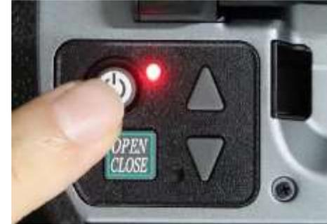
When the power is off but the sheath clamp is open, the wind-protector may not close and the display shows the message below. In this case, please close the sheath clamp and turn off the power by pressing the ON/OFF key.
