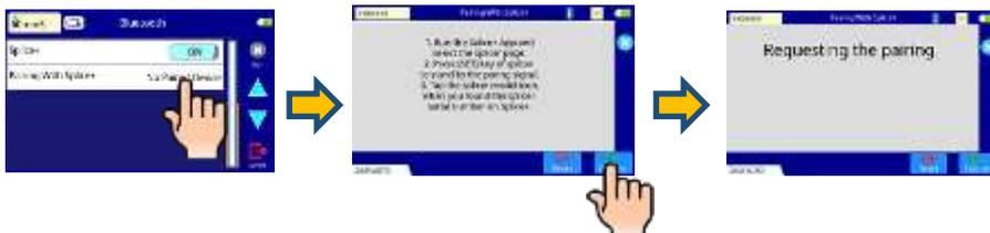
5. Wait until the splicer shown is in the Splice+. Tap the icon. Icon color will change (Light blue), when pairing is finished.
