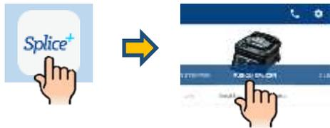
4. Select the [Pairing With Splice+] in the splicer. Then press [Set] key.
