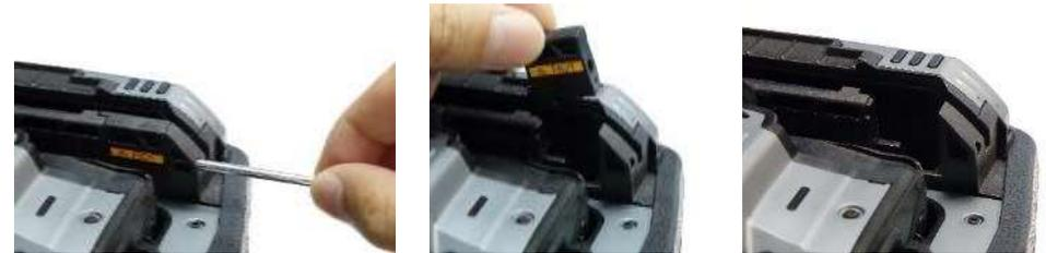
To reinstall, press down on the connector holder from the top so it is secure against the fusion splicer body, and reinsert the screw on the right side.
