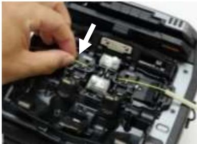
3. Tilt the fiber to slide the protection sleeve toward the left while maintaining tension.
