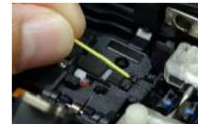
3. Press **[SET]** key to initiate the Fusing Power Calibration.
