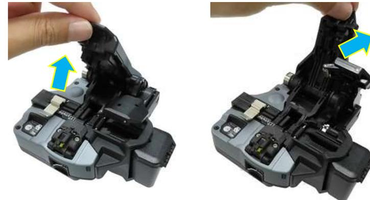
3. Open the lid of the fiber plate AD-10-M24. Set the cleaned fiber onto the fiber plate. Check and adjust the fiber length using the scale on the fiber plate.
