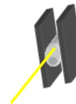
Apply tension until heater holds the fiber.
