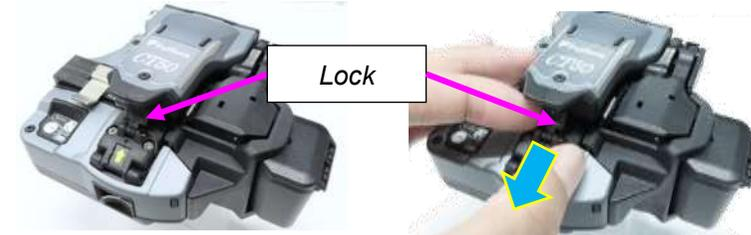
2. Lift the lever until it stops. The blade is automatically set at the start position and is now ready to cleave the fiber.
