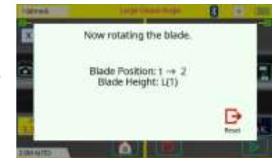
It is easy to detect blade wear by correlating blade positions with cleaving errors given by the splicer. If the splicer detects blade wear by analyzing the fiber image, the splicer sends a command to the cleaver to rotate the blade to the next available unconsumed position. By using this function, it can get the low-splice loss and stability. The splicer informs the operator with an on-screen alarm during rotation the blade.
