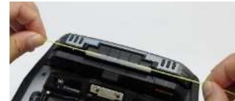
Two-heater plates sandwich the protection sleeve as shown below. Releasing tension earlier may cause the protection sleeve to fall from the proper heating location.
