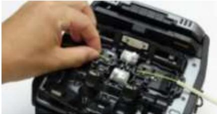
(2) Slide the protection sleeve until it touches your left hand, while holding tension on the splice.
