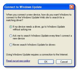
Select either of the first two options to enable Windows Update reconnect your SPC device to a spare USB port. If the PC is connected to the web, the drivers will now load.
