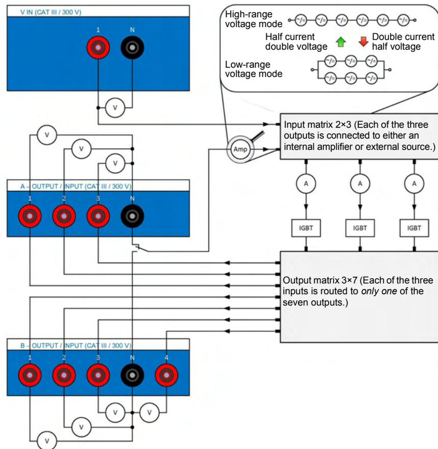
Figure 3-3 The *CIBANO 500* voltage operating mode
