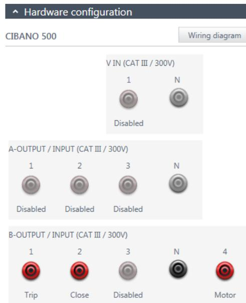
Figure 6-13 Hardware configuration of the Minimum Pickup test
