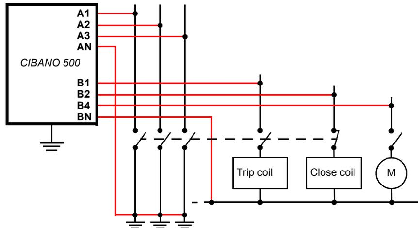
Figure 4-3 Typical measurement setup for the Timing test on medium-voltage circuit breakers with complete disconnection from the station
