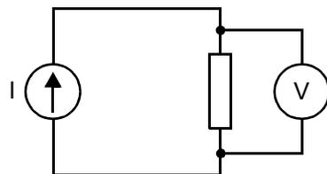
Figure 6-3 Principal scheme of the contact resistance test
