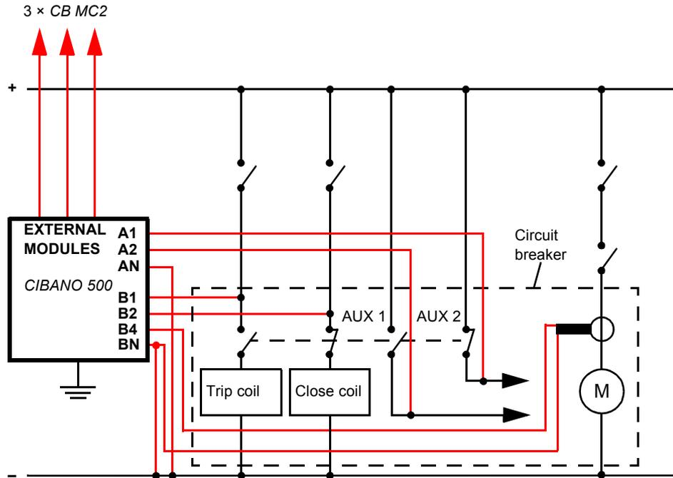
Figure 6-29 Typical measurement setup for the Dynamic Contact Resistance test
