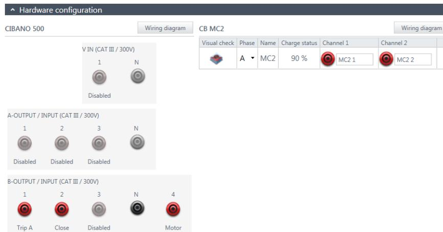
Figure 6-28 Hardware configuration of the Dynamic Contact Resistance test
