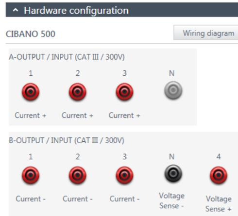
Figure 6-2 Hardware configuration of the Contact Resistance test
