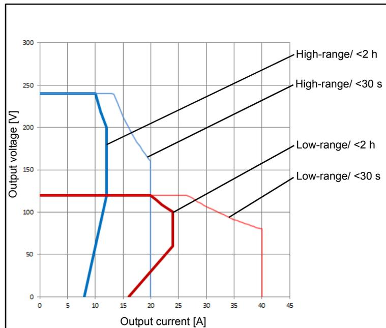
Figure 10-2 AC output characteristics
