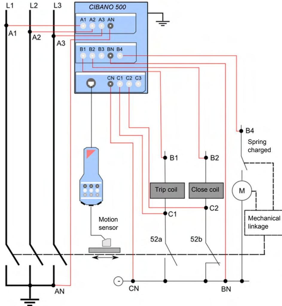
Figure 6-10 Connecting *CIBANO 500* to the circuit breaker for the Timing test
