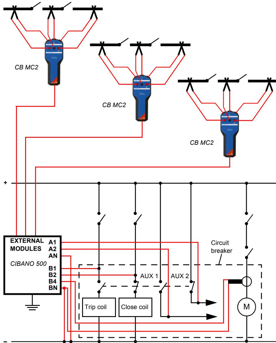
Figure 4-4 Typical measurement setup for testing high-voltage circuit breakers
