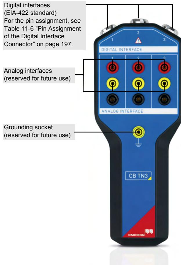
Figure 11-3 Front view of the *CB TN3* module
