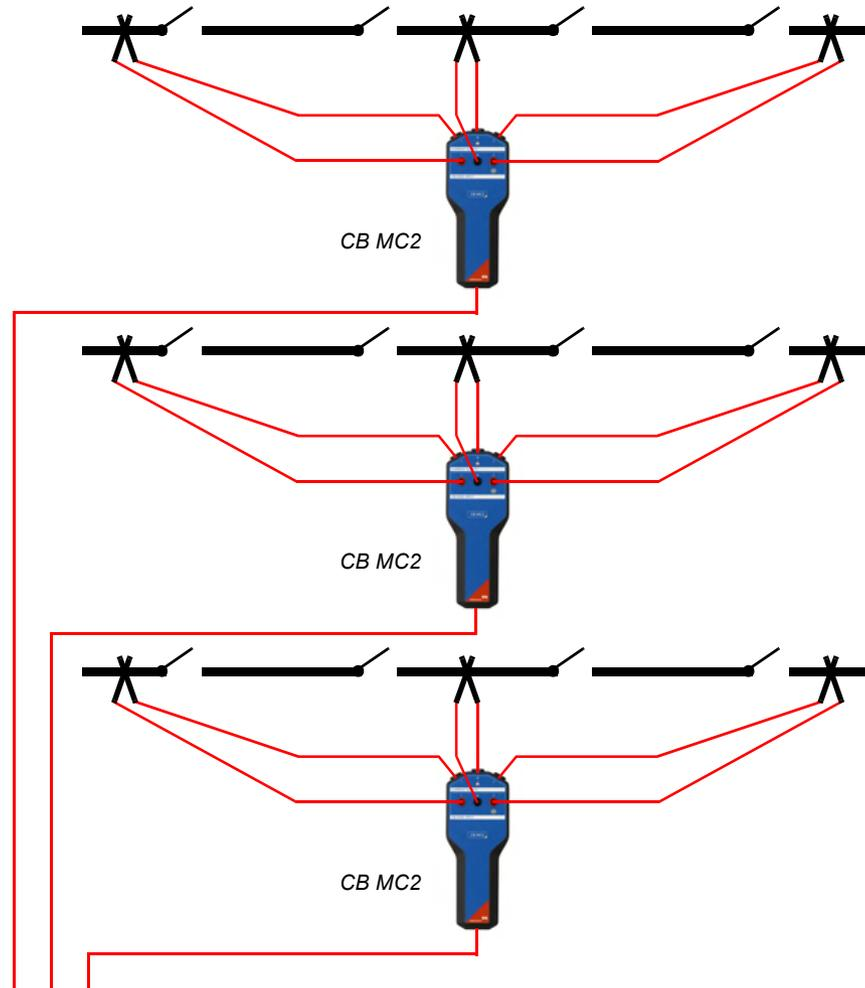
Figure 6-21 Testing the phase synchronicity of the previous example
