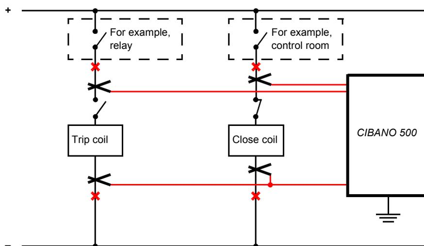
Figure 4-2 Principal connection of *CIBANO 500* to the test object
