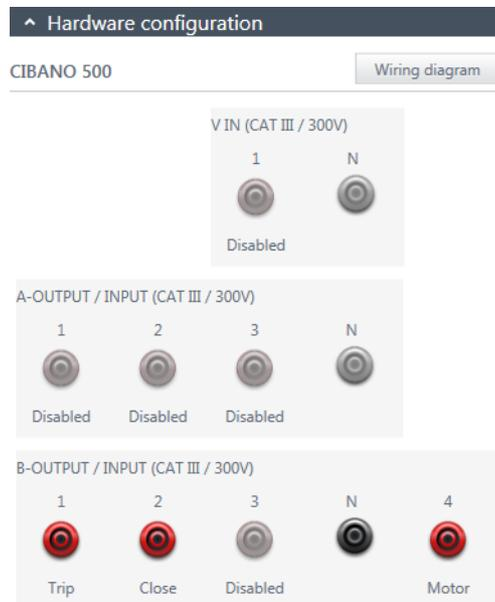
Figure 6-32 Hardware configuration of the Minimum Pickup test
