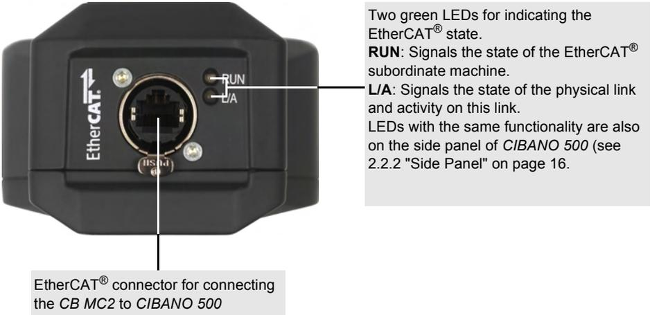
Figure 11-2 Bottom view of the *CB MC2* module
