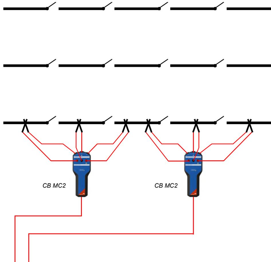
Figure 6-20 Example of the connection to the first phase of a circuit breaker with four interrupters per phase
