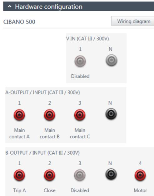
Figure 6-5 Hardware configuration of the Timing test
