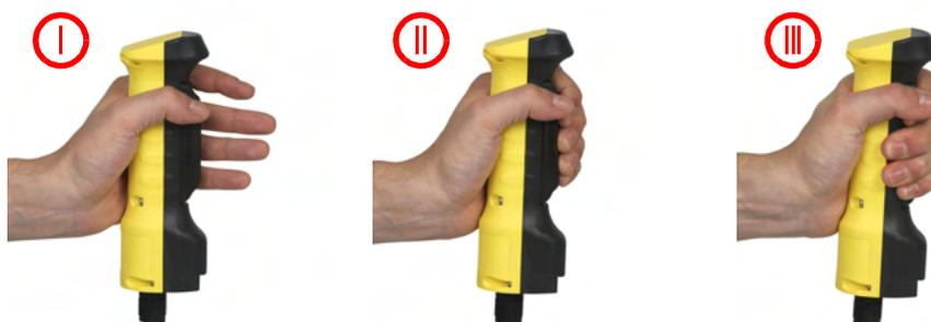
Figure 11-6 Operating positions of the *3-Position Remote Safety Switch*
