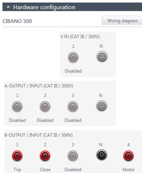
Figure 6-15 Hardware configuration of the Motor Current test
