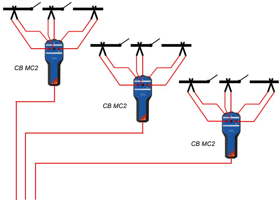
Figure 6-19 High-voltage section of a circuit breaker with two interrupters per phase with connected *CB MC2* modules
