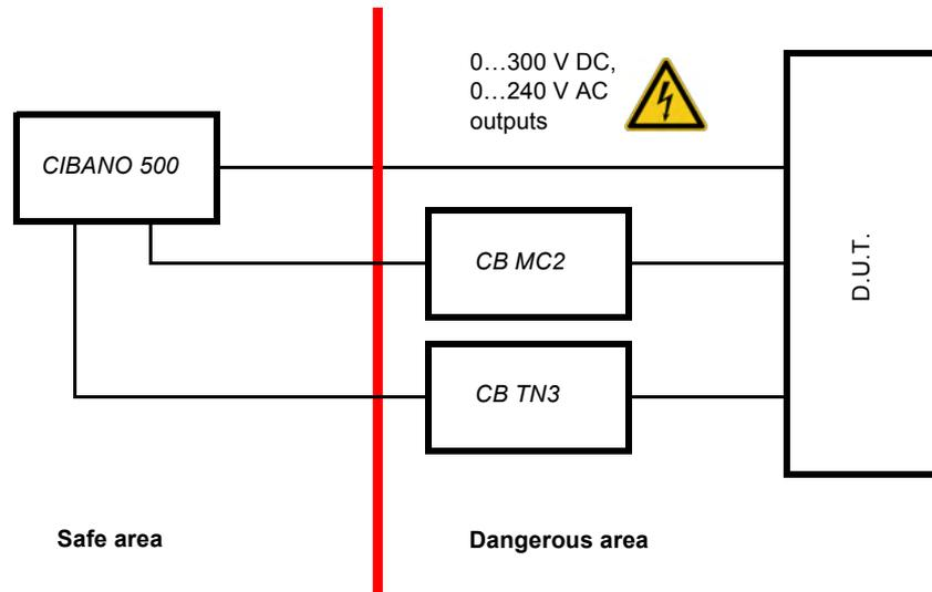
Figure 1-1 Example of the separation of the safe and dangerous areas
