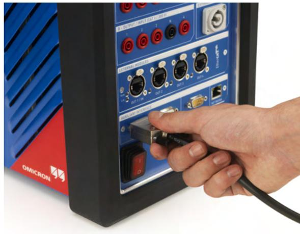
Figure 11-7 Connecting the *3-Position Remote Safety Switch* to the test system
