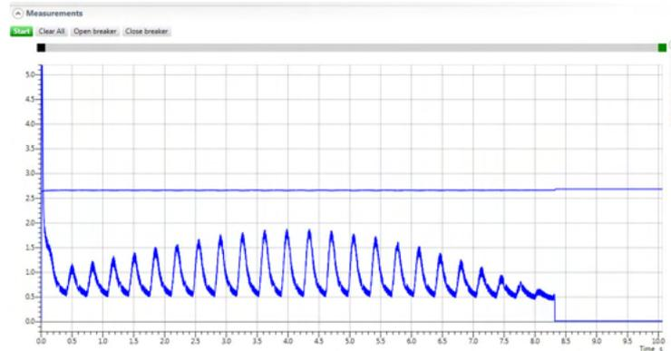
Figure 6-17 Example of the Motor Current test results
