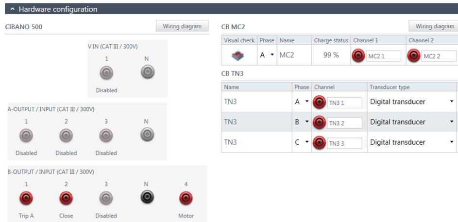
Figure 6-38 Example of the hardware configuration of the Dynamic Contact Resistance test for measuring the main contact travel during operation
