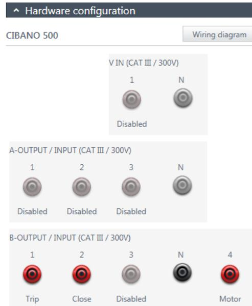
Figure 6-34 Hardware configuration of the Motor Current test
