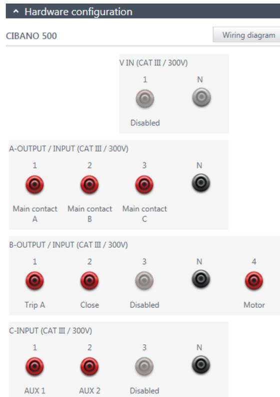
Figure 6-9 Hardware configuration of the Timing test
