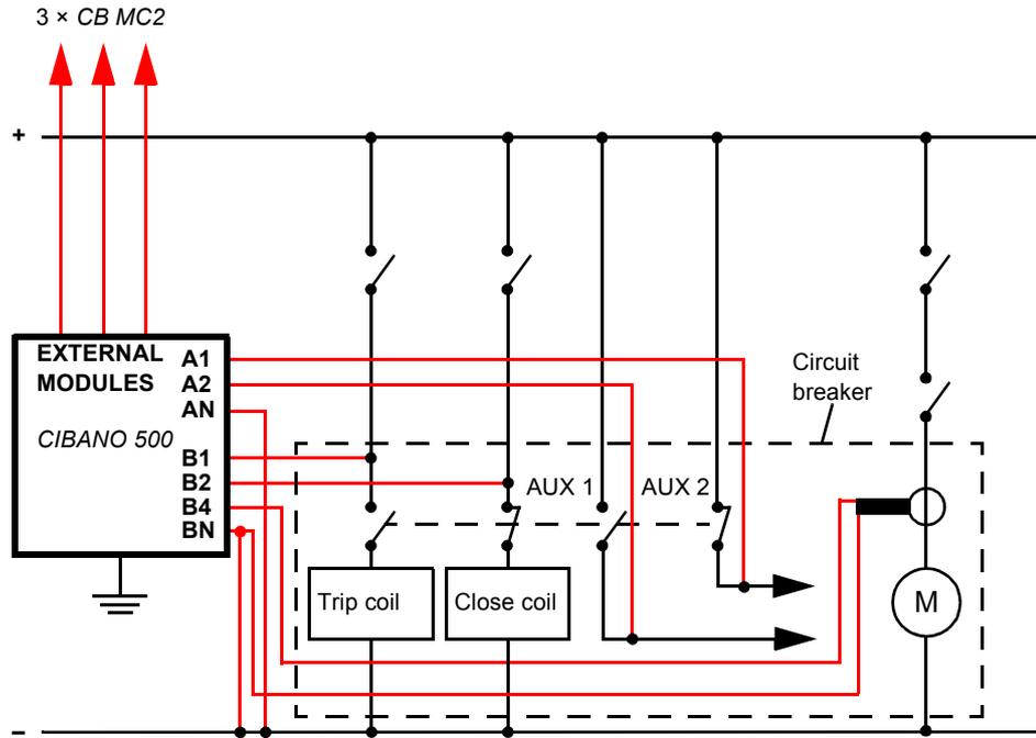
Figure 6-25 Typical measurement setup for the Timing test
