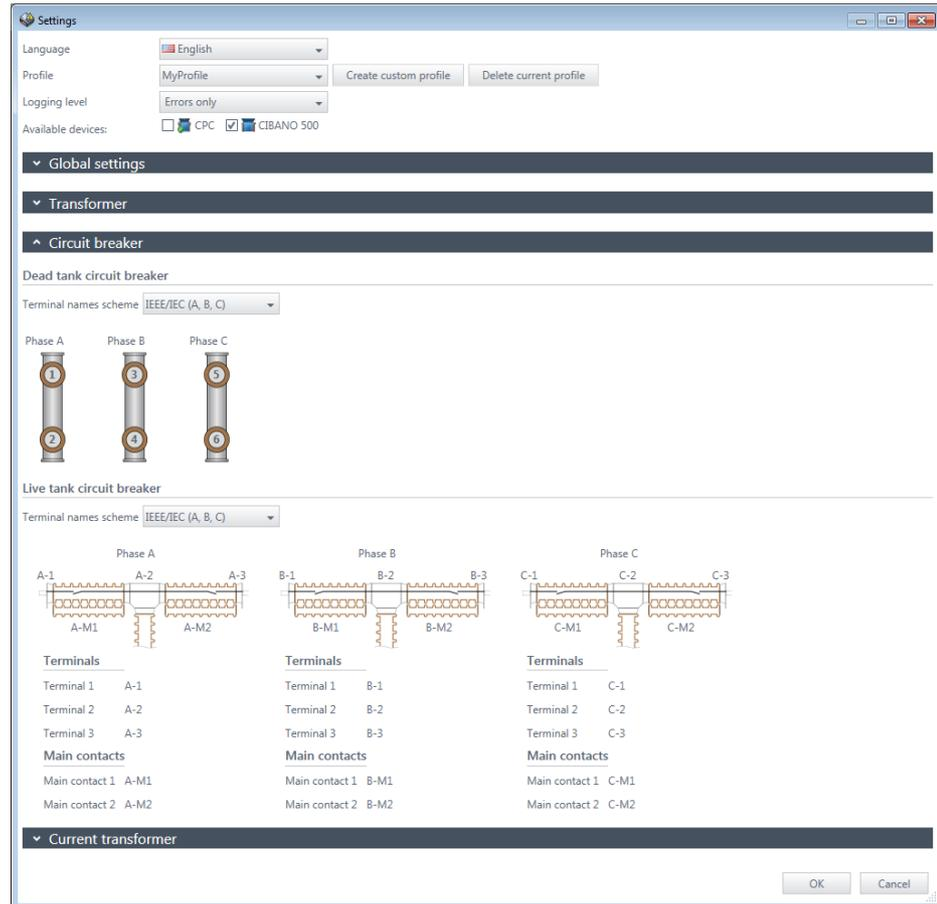
Figure 5-5 **Settings** dialog box: circuit breaker area
