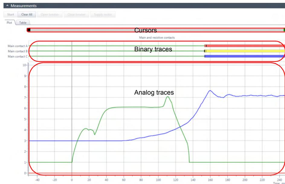
Figure 5-13 Example of the graphical display of measurement data
