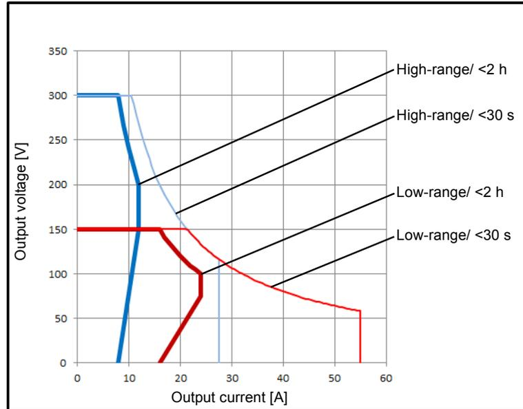
Figure 10-1 DC output characteristics
