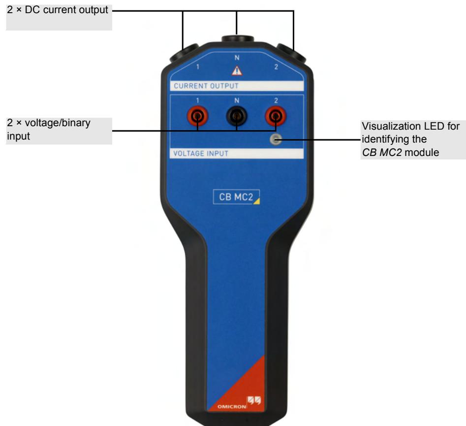
Figure 11-1 Front view of the *CB MC2* module
