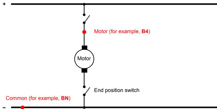
Figure 6-35 Connecting *CIBANO 500* to the circuit breaker for the Motor Current test (The end position switch opens when the spring is charged.)
