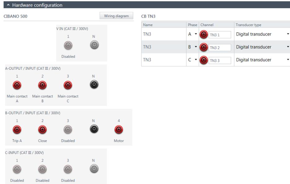
Figure 6-37 Example of the hardware configuration of the Timing test for measuring the main contact travel during operation
