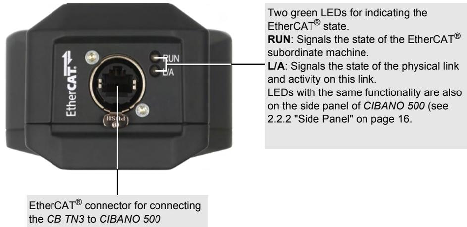
Figure 11-4 Bottom view of the CB TN3 module
