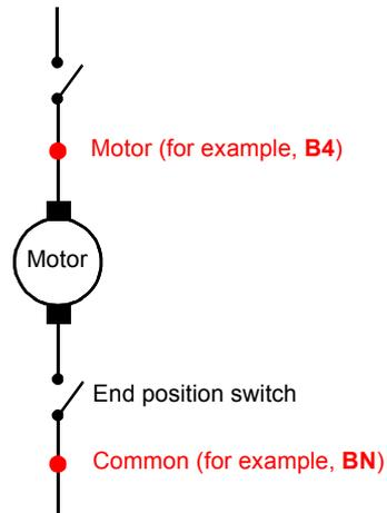
Figure 6-16 Connecting *CIBANO 500* to the circuit breaker for the Motor Current test (The end position switch opens when the spring is charged.)
