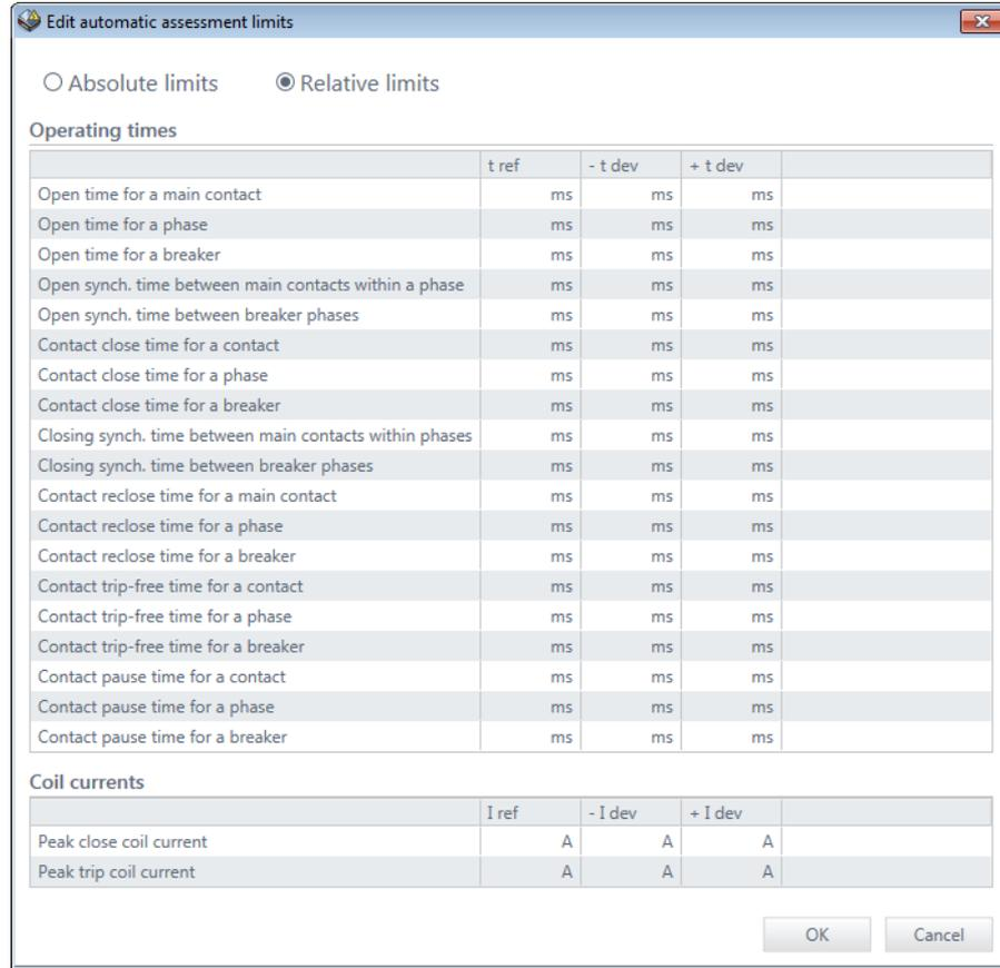
Figure 6-8 Edit automatic assessment limits dialog box: relative limits
