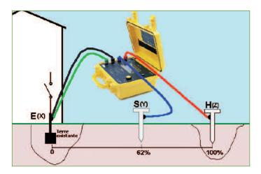
The 4P measurement method is more accurate and can be used to measure low earth resistances. The results obtained with this measurement method are ideal for the requirements of energy distributors such as EDF.
