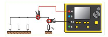
earth measurements using the classic 3P - R1 & R2 method, and 1 earth measurement using the 2P - R1-2 method. The instrument then **automatically** calculates the coupling resistance: Rc = (R1 + R2 - R1-2) / 2.
