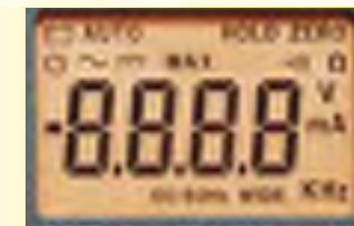
Backlit 10 000 counts LCD screen
