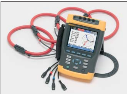
Fluke 435 with flex clamps
