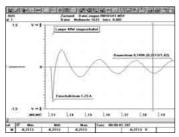
Rapid changes to measurement values can be recorded with METRAHit®22M/26M and 29S instruments at sampling rates of 1 kHz and 2 kHz respectively.
