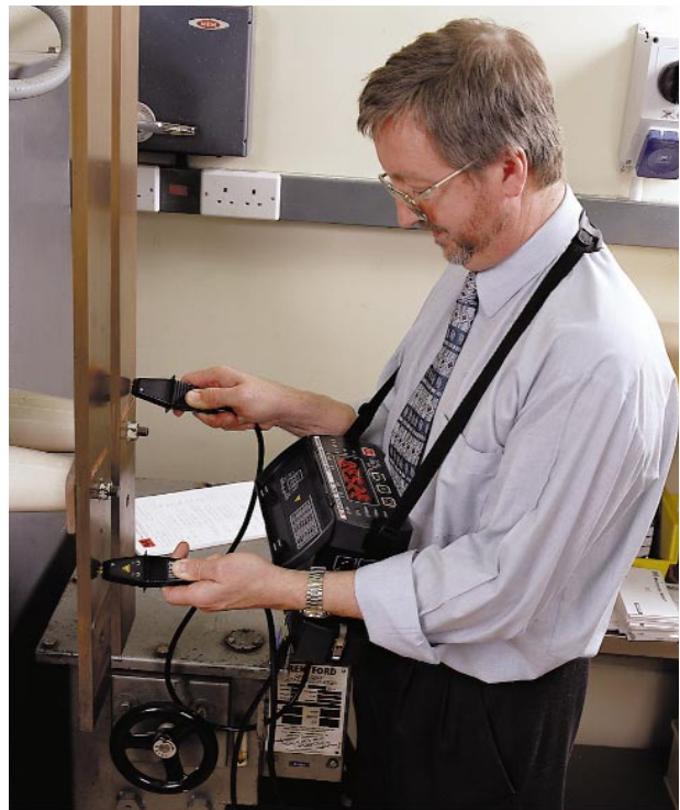
The DLROs are light enough to be worn around the neck. They are also small enough to be taken into areas which were previously too cramped for easy testing.
