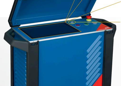
The USB interface can be used to import and export test files to and from TESTRANO 600.
