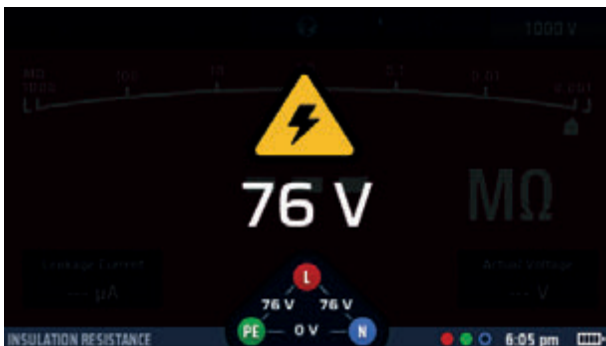
Fig 11: Insulation live circuit warning
