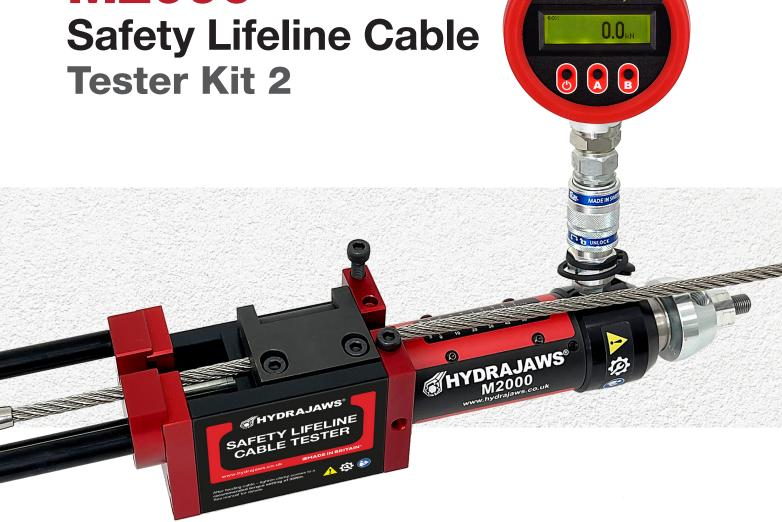
The Hydrajaws M2000 Safety Lifeline Cable Tester KIT 2 is a complete kit enabling engineers to validate the strength of swaged components on newly installed or existing engineered lifeline systems to ensure compliance with BS 7883 up to a maximum tensile load of 25kN.
