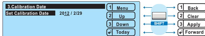
When the calibration date setup screen is displayed, pressing SHIFT changes the functions of the keys.
