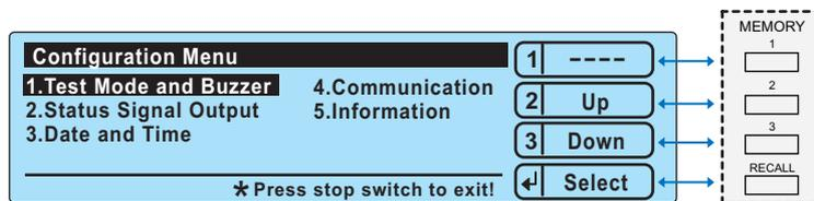
If you display a configuration item setup menu from the Configuration Menu, functions such as Menu, Up, Down, Check, and Apply are assigned to the MEMORY keys.
