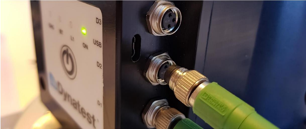
Connect the additional geophones to the connectors on the right side of the electronics box. It is very important that geophone number 2 is connected to D2 and geophone number 3 to D3. Each plug should be pressed in until it locks with a click (to later disconnect, pull the plug body, NOT the cable!!)
