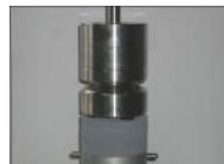
9. Screw the lower part of the Weight Guide Shaft (the one with engraved drop height Nos 1 to 11, No. 11 upwards) into the top stem of the LWD Main Unit.
