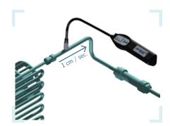
For optimum leak detection, hold the sensor head (3) as close as possible over the air-conditioning pipe. Move the sensor head slowly along the air-conditioning pipe (max. 1 cm per second).
