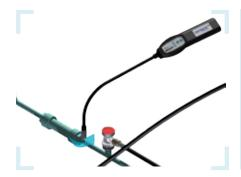
Screwed unions or other connection points must be "scanned" slowly, i.e. move the sensor head (3) right around the complete connection point.
