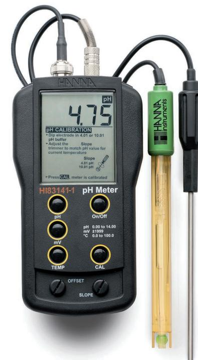
7. Wait a few minutes and use the calibration screwdriver to adjust the OFFSET trimmer until it displays the pH value at the previously noted temperature. See pH Buffer Values at Various Temperatures table.
