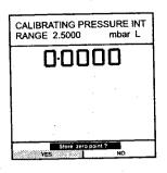
Apply fourth calibration pressure (positive half full scale) and store the half FS point as shown below (e.g.),
