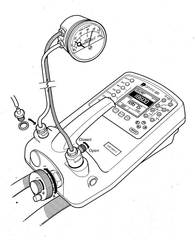
Figure B2 - DPI 610LP Test Connections
