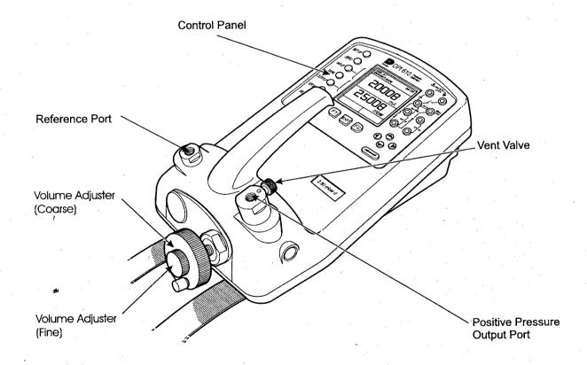
Figure B1 - DPI 610LP Calibrator Controls
