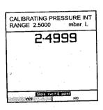
After application of the final calibration pressure, the calibration results are displayed as shown below. To view the second page of calibration data press MORE (F1). Press ENTER complete the pressure calibration procedure.
