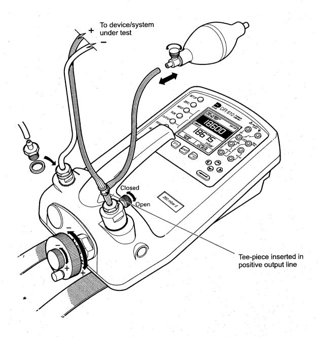
Figure B3 - DPI 610LP Hand Pump Connections
