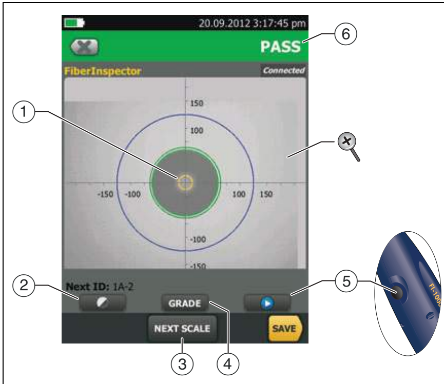
Figure 39. FiberInspector Image with Manual Grading Selected
