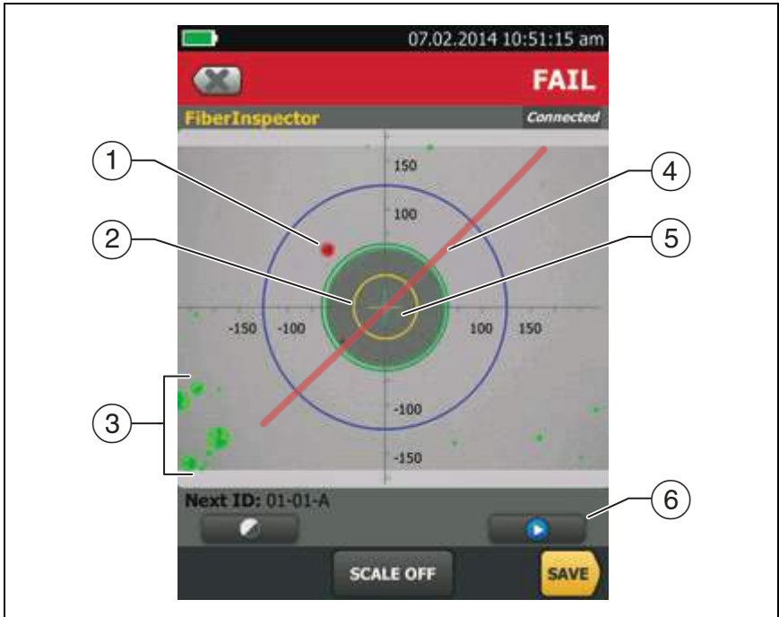
Figure 40. FiberInspector Image with Defect Analysis
