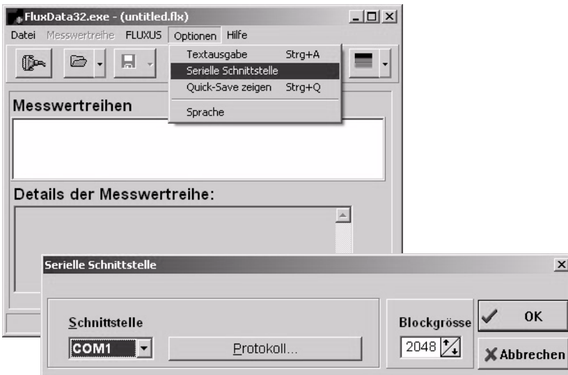
Fig. 12.1: Selection of the serial interface
