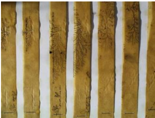
Electrical Trees in PILC Paper Insulation
